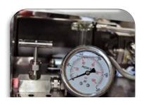
4. Fully open the pressure regulating valve next to the pressure gauge by turning it *counter clockwise* until fully open.
