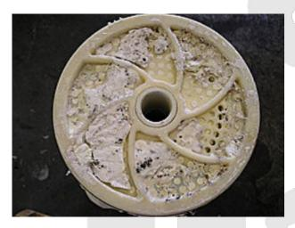
Mineral fouling is a slow gradual process in seawater systems but can occur much faster in groundwater systems that have high mineral content. In this situations it is advised to have a regular cleaning schedule to ensure that the fouling of the membranes is kept in check. Depending on your site this may be as often as fortnightly or quarterly.
