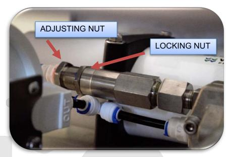
NOTE: that when the pressure relief valve releases water will shoot out of the valve, this will drop the pressure of your system
