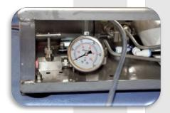
8. Slowly increase the system operating pressure by turning the pressure regulating valve in a clockwise direction. Slowly increase the system pressure up to 600 PSI. Allow the pump and motor assembly to run at 600 PSI for a ten-minute breakin period. NOTE: You will observe fresh water starting to flow through the flowmeter once you reach approximately 600-650 PSI.
