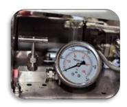
**CAUTION**: Do not run freshwater through the RO pressure vessel at high pressure; always make sure the pressure regulating valve is completely open (turn counter clockwise until the valve stops). Running fresh water through the RO membranes at high pressure will rupture the membrane and destroy it
