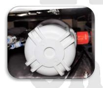
4 Leaning unit on its side unscrew the filter housing and empty water from the housing and from the hoses.
