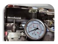
4. Fully open the pressure regulating valve next to the pressure gauge by turning it *counter clockwise* until fully open.
